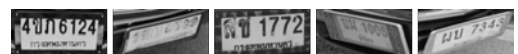
Fig. 7 Samples of Thai license plates with blur, side-view distortion, and stroke-level confusion.
