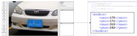
Fig. 4 License plate annotation using LabelImg with bounding box saved in XML format.
